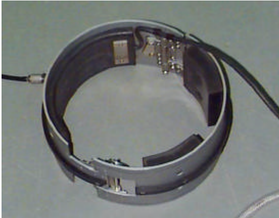
Bladder Track shown with collar partially open
