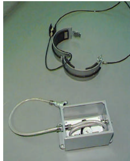
Bladder Track & Junction Box
