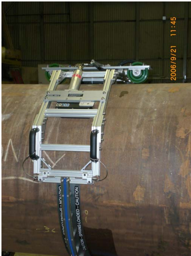
Scanner on mock-up in Alaska
