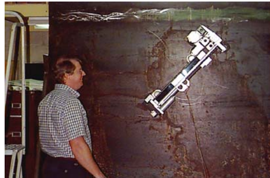
Navigator on BWR OD mockup plate observed by Design Engineer, Jay Baldwin
